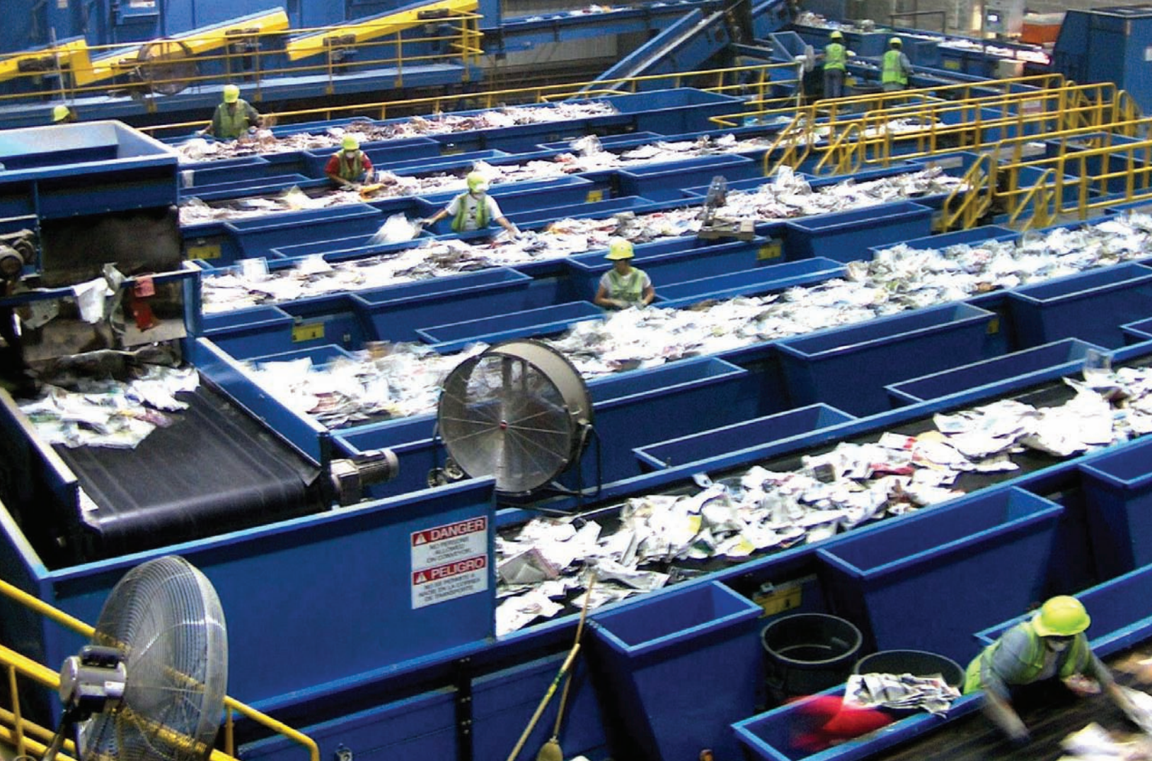
On the 'pre-sort' line at a plant operated by Waste Management Recycle America, workers pick through conveyor belts of garbage to pluck out materials that can't be recycled.
